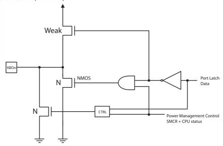
The current limitation of the CTRL block requires a polarisation current of about 250µA. This block is automatically disabled in power-down, power-save, standby and extended standby modes.
