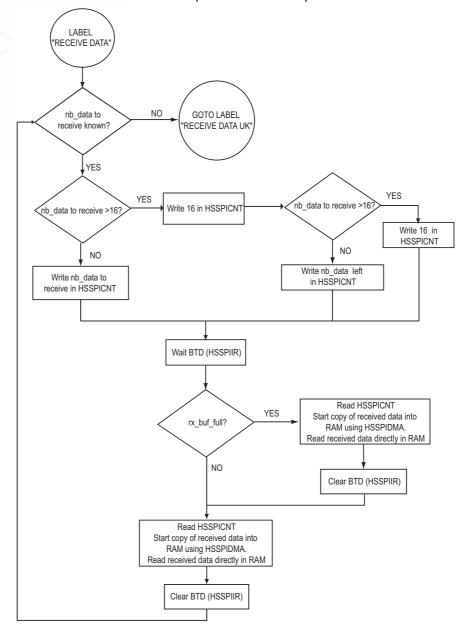
Figure 21-7. SPI - Slave with DPRAM operation - Second part
