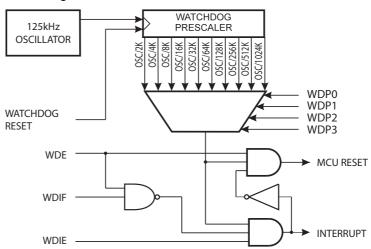
The Watchdog Timer (WDT) is a timer counting cycles of a separate on-chip 125 kHz oscillator. The WDT gives an interrupt or a system reset when the counter reaches a given time-out value. In normal operation mode, it is required that the system uses the WDR - Watchdog Timer Reset - instruction to restart the counter before the time-out value is reached. If the system doesn't restart the counter, an interrupt or system reset will be issued.
