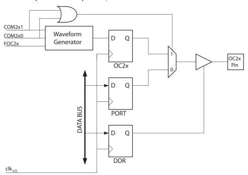
The general I/O port function is overridden by the Output Compare (OC2x) from the Waveform Generator if either of the COM2x1:0 bits are set. However, the OC2x pin direction (input or output) is still controlled by the Data Direction Register (DDR) for the port pin. The Data Direction Register bit for the OC2x pin must be set as output before the OC2x value is visible on the pin. The port override function is independent of the Waveform Generation mode.
