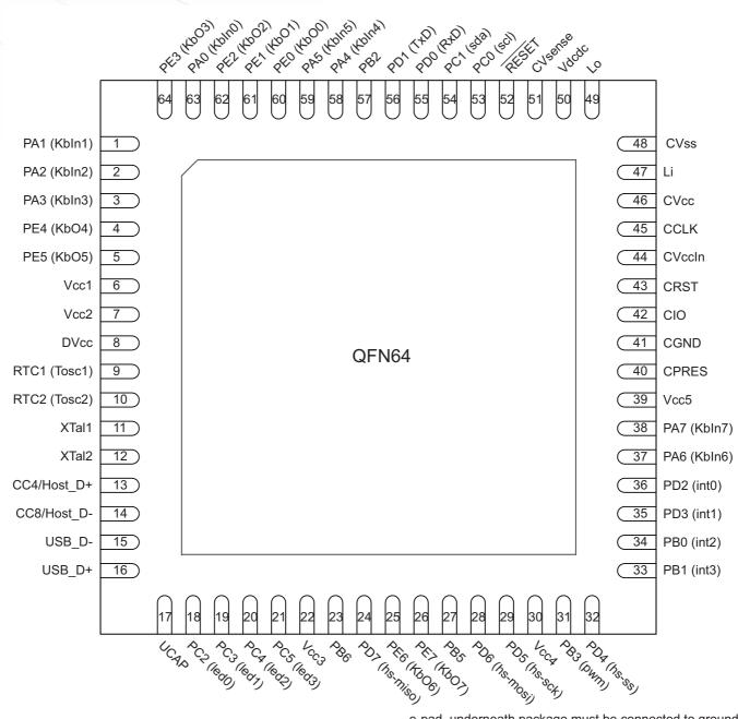
e-pad, underneath package must be connected to ground
