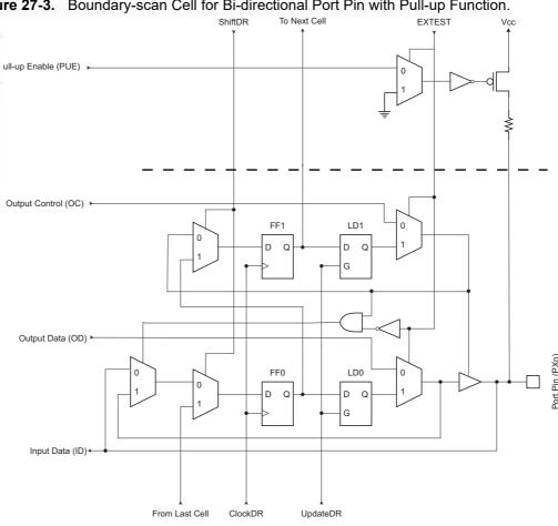
Figure 27-3. Boundary-scan Cell for Bi-directional Port Pin with Pull-up Function.
