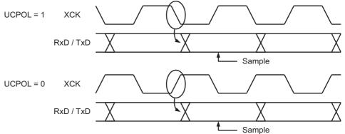
The UCPOL0 bit UCRSC selects which XCK clock edge is used for data sampling and which is used for data change. As Figure 18-3 shows, when UCPOL0 is zero the data will be changed at rising XCK edge and sampled at falling XCK edge. If UCPOL0 is set, the data will be changed at falling XCK edge and sampled at rising XCK edge.
