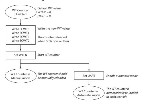
To reload the WT counter, SCICR.WTEN bit should be cleared before writing a new value in SCWT registers. Then the counter will be enabled by setting SCICR.WTEN bit.
