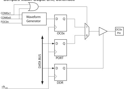
The general I/O port function is overridden by the Output Compare (OC0x) from the Waveform Generator if either of the COM0x1:0 bits are set. However, the OC0x pin direction (input or output) is still controlled by the Data Direction Register (DDR) for the port pin. The Data Direction Register bit for the OC0x pin (DDR\_OC0x) must be set as an output before the OC0x value is visible on the pin. The port override function is independent of the Waveform Generation mode.
