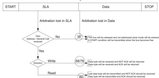
Figure 22-21. Possible Status Codes Caused by Arbitration
