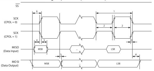
Figure 31-3. SPI Interface Timing Requirements (Slave Mode)
