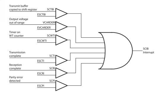
This signal is high level active. Each of the sources is able to activate the SCIB interruption which is cleared by software by clearing the corresponding bits in the Smart Card Interrupt register.
