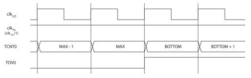
Figure 13-9 shows the same timing data, but with the prescaler enabled.
