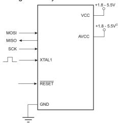
When programming the EEPROM, an auto-erase cycle is built into the self-timed programming operation (in the Serial mode ONLY) and there is no need to first execute the Chip Erase instruction. The Chip Erase operation turns the content of every memory location in both the Program and EEPROM arrays into \$FF.
