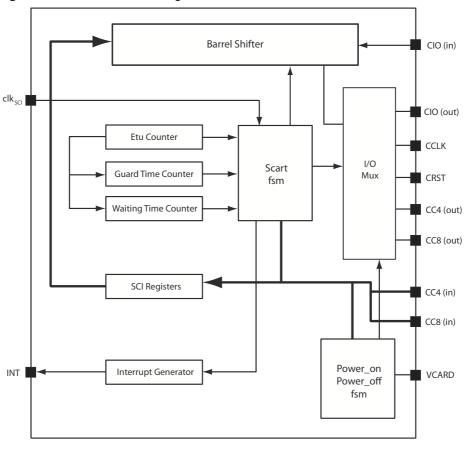
Figure 15-1. SCIB Block Diagram
