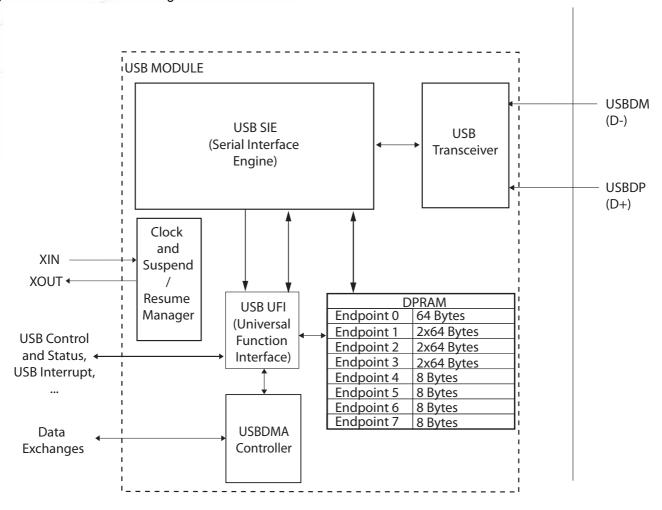
The USB module of the AT90SCR100/200 is made up of the following elements:
