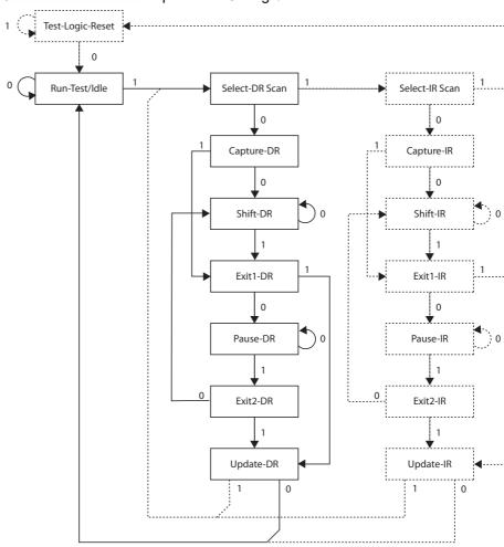
Figure 29-7. State Machine Sequence to Change/Read the Data Word
