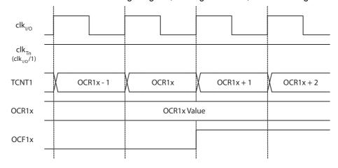
Figure 13-22 shows the same timing data, but with the prescaler enabled.
