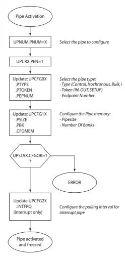
Once the Pipe is activated (UPCRX.PEN set), the hardware is ready to send requests to the Device.
