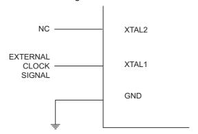
When this clock source is selected, start-up times are determined by the SUT Fuses as shown in Table 7-4.
