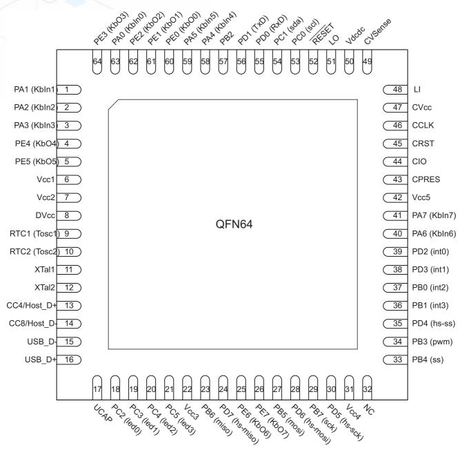
e-pad, underneath package must be connected to ground NC: Not Connected (pin 32)
