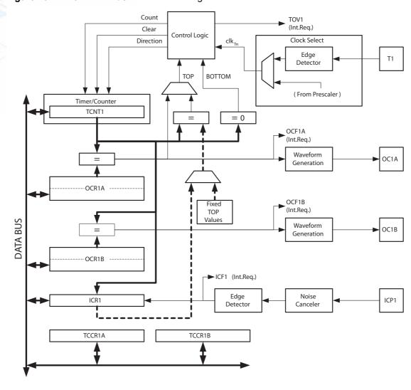
Figure 13-12. 16-bit Timer/Counter Block Diagram
