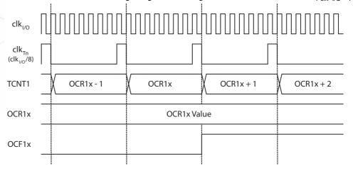
Figure 13-23 shows the count sequence close to TOP in various modes. When using phase and frequency correct PWM mode the OCR1x Register is updated at BOTTOM. The timing diagrams will be the same, but TOP should be replaced by BOTTOM, TOP-1 by BOTTOM+1 and so on. The same renaming applies for modes that set the TOV1 Flag at BOTTOM.
