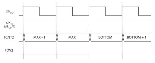
Figure 13-33 shows the same timing data, but with the prescaler enabled.
