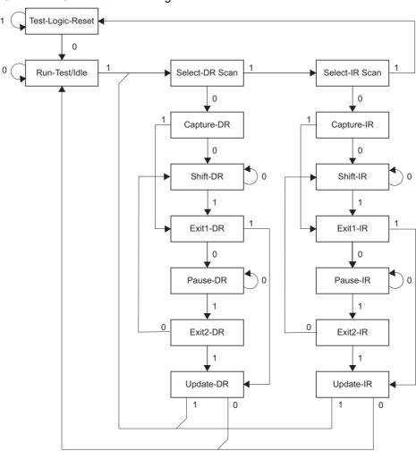
Figure 26-2. TAP Controller State Diagram
