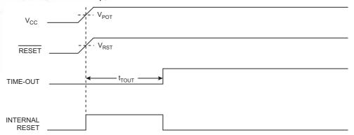
Figure 9-3. MCU Start-up, RESET Extended Externally
