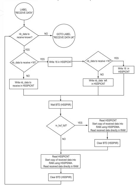
Figure 19-7. SPI - Slave with DPRAM operation - Second part
