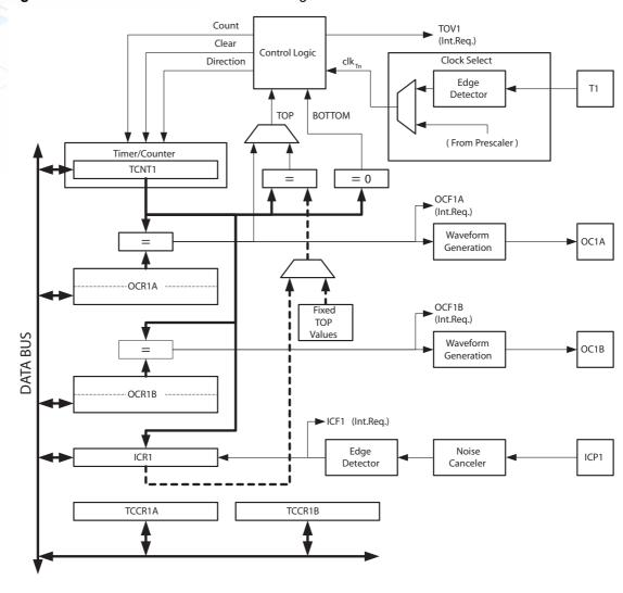
Figure 13-12. 16-bit Timer/Counter Block Diagram
