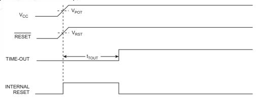
Figure 9-3. MCU Start-up, RESET Extended Externally
