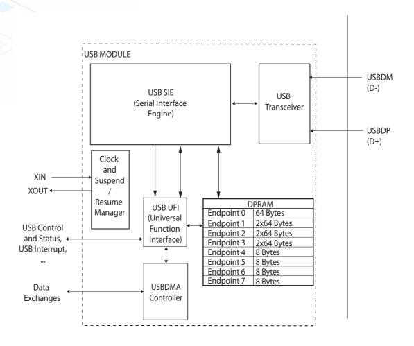
The USB module of the AT90SCR400 is made up of the following elements:
