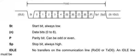
The frame format used by the USART is set by the UCSZ02:0, UPM01:0 and USBS0 bits in UCSR0B and UCSR0C. The Receiver and Transmitter use the same setting. Note that changing the setting of any of these bits will corrupt all ongoing communication for both the Receiver and Transmitter.
