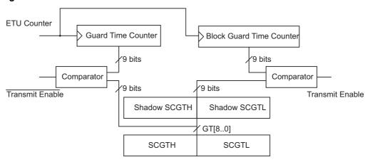
To illustrate the use of Guard Time and Block Guard Time, consider the ISO/IEC 7816-3 recommendation: Guard Time = 2 (minimum delay between 2 consecutive characters sent by the Terminal = 12 ETUs) and Block Guard Time = 22 ETUs.
