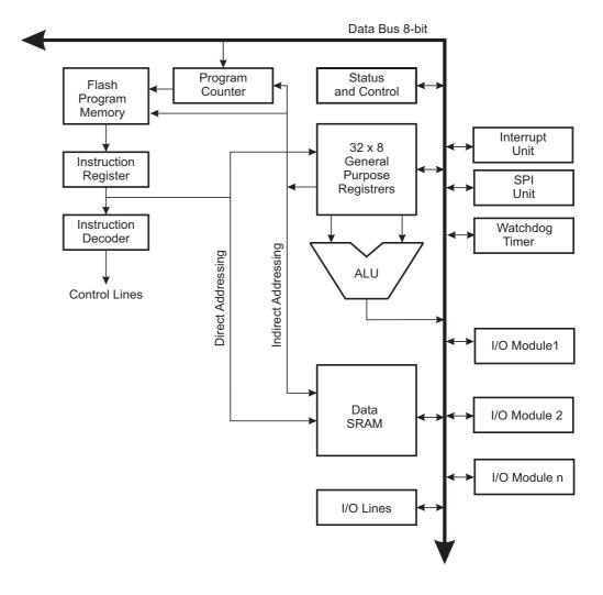
In order to maximize performance and parallelism, the 8/16-bit RISC CPU uses a Harvard architecture – with separate memories and buses for program and data. Instructions in the program memory are executed with a single level pipelining. While one instruction is being executed, the next instruction is pre-fetched from the program memory. This concept enables instructions to be executed in every clock cycle. The program memory is In-System Reprogrammable Flash memory.
