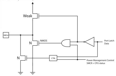
The current limitation of the CTRL block requires a polarisation current of about 250µA. This block is automatically disabled in power-down, power-save and standby modes.
