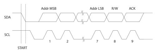
Figure 20-4. Address Packet Format
