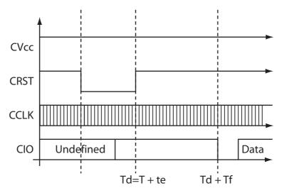
The removal of the smart card will automatically start the power off sequence as described in Figure 15-13.
