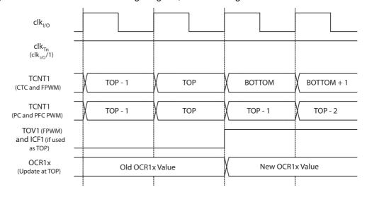
Figure 13-24 shows the same timing data, but with the prescaler enabled.
