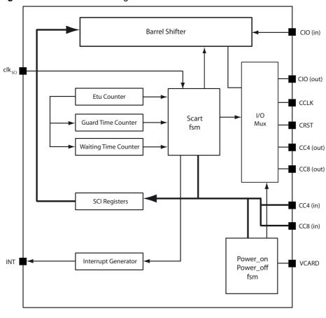
Figure 15-1. SCIB Block Diagram
