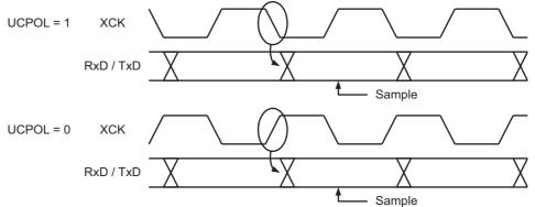
The UCPOL0 bit UCRSC selects which XCK clock edge is used for data sampling and which is used for data change. As Figure 17-3 shows, when UCPOL0 is zero the data will be changed at rising XCK edge and sampled at falling XCK edge. If UCPOL0 is set, the data will be changed at falling XCK edge and sampled at rising XCK edge.
