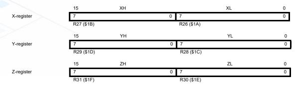
In the different addressing modes these address registers have fixed displacement, automatic increment, and automatic decrement functionality (see the instruction set reference for details).
