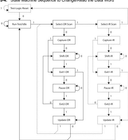
Figure 25-4. State Machine Sequence to Change/Read the Data Word
