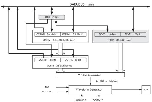
Figure 13-15. Output Compare Unit, Block Diagram
