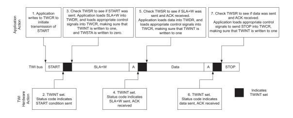
1. The first step in a TWI transmission is to transmit a START condition. This is done by writing a specific value into TWCR, instructing the TWI hardware to transmit a START condition. The value to write is described later on. However, it is important that the TWINT bit is set in the value written. Writing a one to TWINT clears the flag. The TWI will not start any operation as long as the TWINT bit in TWCR is set. Immediately after
