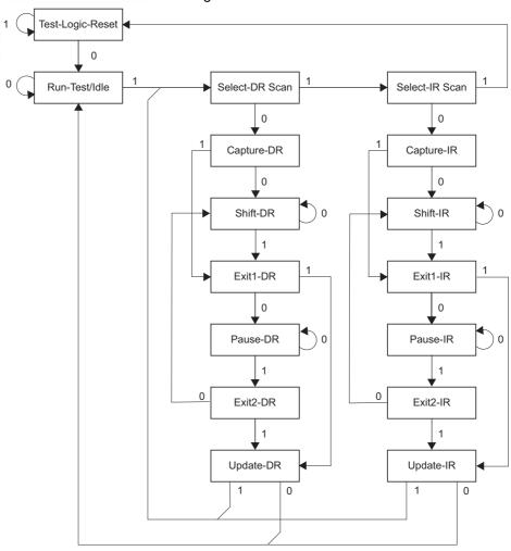
Figure 22-2. TAP Controller State Diagram
