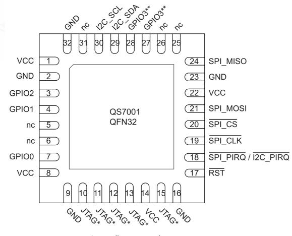
nc = not internally connected \* JTAG is for devt. chips only \*\* double bonding of GPIO3
